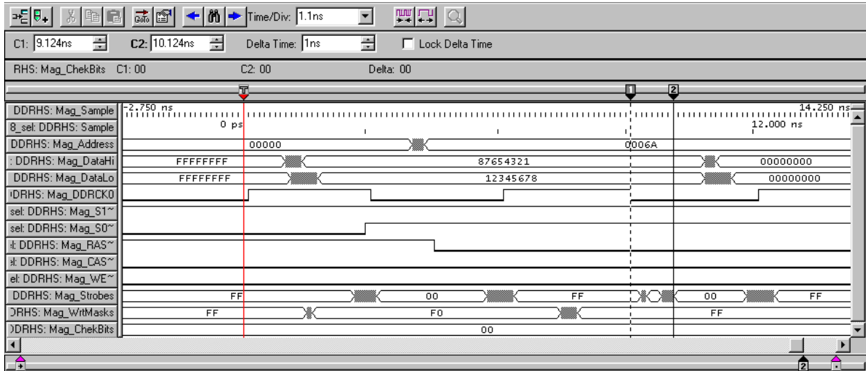
Figure 9- Measuring DDRHSM Write Data Setup & Hold
