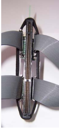
Top view of PCIINTR module with P6960 probes connected and Velcro attached. Note the probes are not pulled in toward the PCIINTR module.
