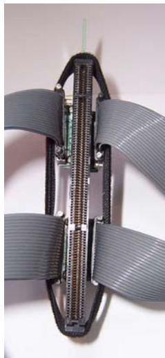
Figure 2- Top view of PCIINTR module with P6960 probes connected and velcro attached Note the probes are not pulled in toward the PCIINTR module.
