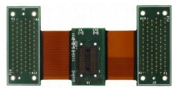
reconstruct 8-, 16-, or 32-bit data buses. Two x16 interposers can be used together to reconstruct 32-bit data buses.
