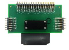
2) Access to oscilloscope probe points where high fidelity measurements can be made at the memory component
