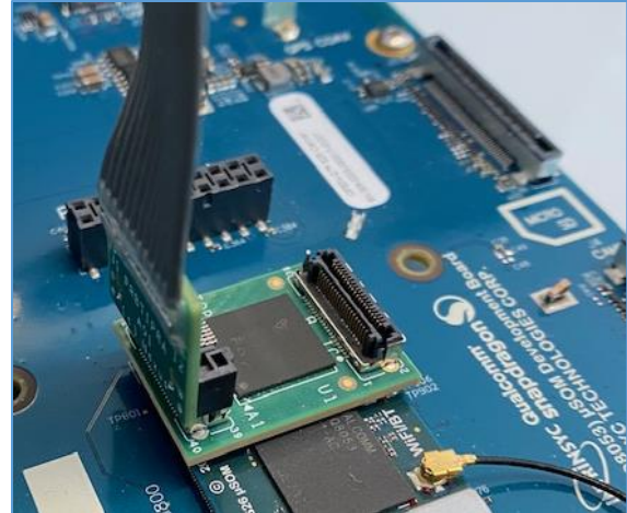
Figure 1 MA 5100 interposer installed under a memory component
