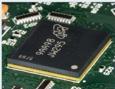
Figure 3 - Side view (photo) of PoP memory soldered onto a processor
