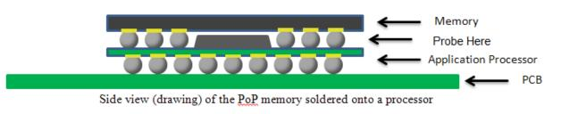
Figure 2 - Side view (drawing) of the PoP memory soldered onto a processer
