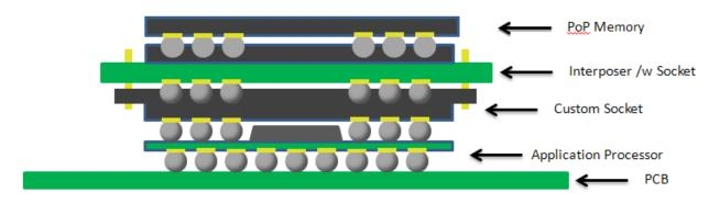
Figure 3 - Side view of the complete interposer installation
