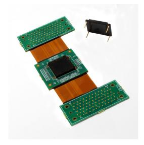
Nexus Technology recommends LPDDR2 component interposers for applications requiring optimal digital validation of LPDDR2 targets. These interposers allow for logic analyzer acquisition of command, address, and data of 168-ball LPDDR2 components. These interposers are also compatible with the Nexus MCA Instrument.
