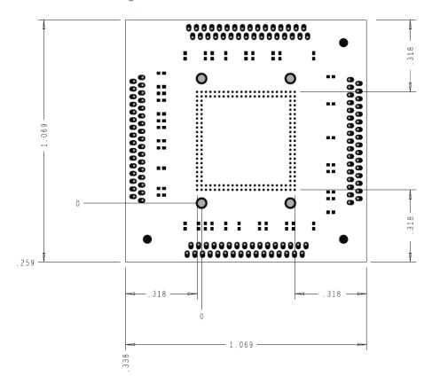
Figure 8: LPDDR2 168-Ball PoP Oscilloscope Component Interposer Dimensions
