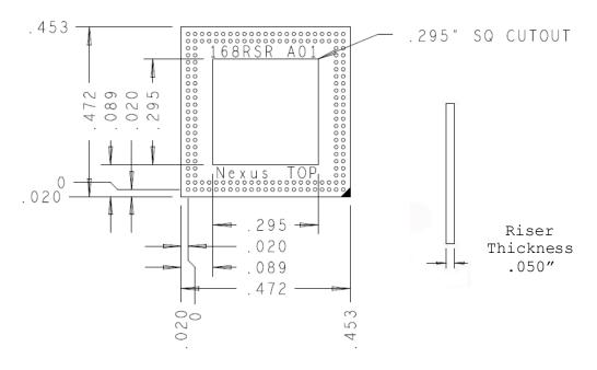
Figure 7: LPDDR2-168 ball Riser Dimensions
