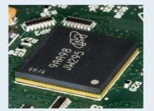
Figure 1 - Side view (photo) of PoP memory soldered onto a processor
