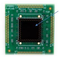
Memory Socket installed. A socket on the interposer provides the ability to quickly and easily change memory components in a target. Simply remove and insert different memory components to validate multiple memory vendors devices.
