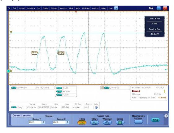
Figure 6: Strobe as seen using the Oscilloscope Component Interposer
