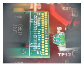
Figure 5 - Soldered down probe tips
