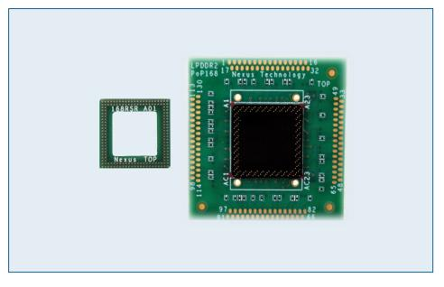
This Memory Component Interposer (MCI) BGA adapter has been designed to provide a high fidelity, easy to probe adapter that connects between your target Board and your memory component. Memory Component Interposers compliment the oscilloscope adapters providing a complete debug solution.
