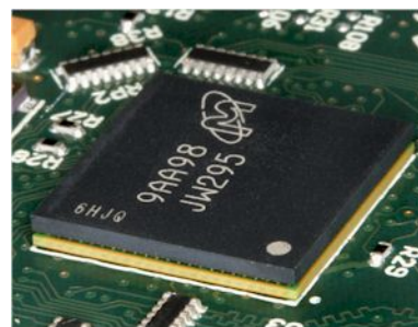
Figure 1 - Side view (photo) of PoP memory soldered on to a processor
