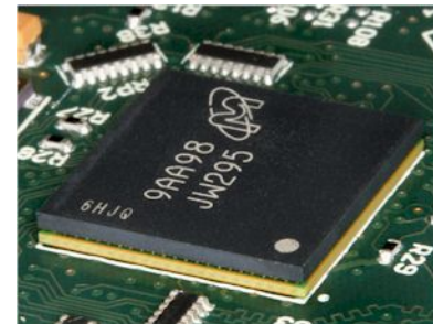
Figure 1: Side view (photo) of PoP memory soldered on to a processor
