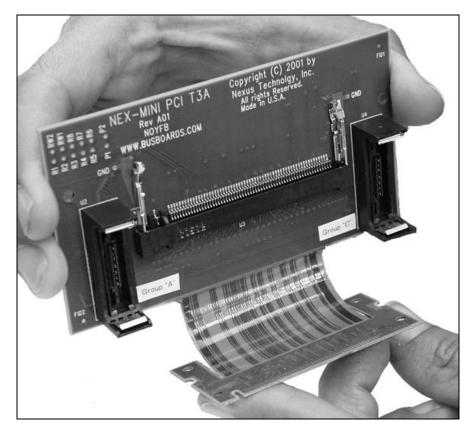
The NEX-MINIPCIT3A is a rigid/flex/rigid design that allows for the mechanical clearance necessary to connect to the target.
