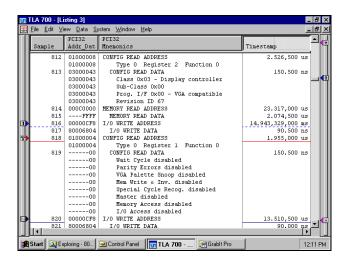
Mini-PCI cycles are identified and Config cycles are decoded. Device information is translated according to Class, sub-Class and Type.
