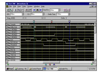
125ps acquisition on each channel provides excellent timing analysis. Each channel is labeled with the appropriate Mini-PCI signal name. Bus format display of grouped signals shown.
