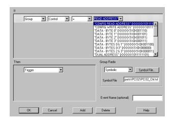
Trigger on pre-defined PCI cycles
