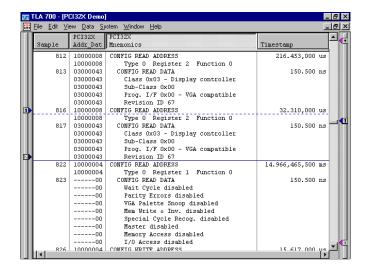
Same disassembly display with Memory and I/O cycles supressed.
