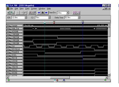
125ps acquisition on each channel provides excellent timing analysis. Each channel is labeled with the appropriate PCI signal name. Bus format display of grouped signals shown.
