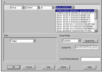
PCI cycles are identified and Config cycles are decoded. Device information is translated according to Class, sub-Class, and Type.
