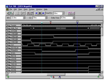
125ps acquisition on each channel provides excellent timing analysis. Each channel is labeled with the appropriate PCI signal name. Bus format display of grouped signals shown.
