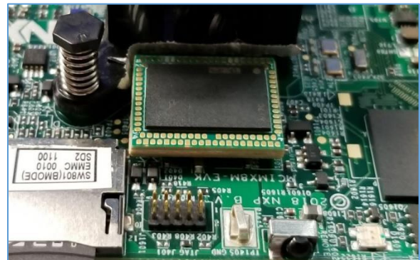
Figure 1 - Direct Attach interposer installed under a memory component
