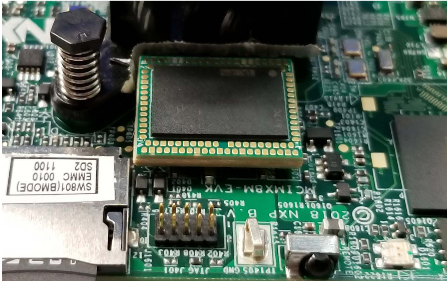
Nexus LPDDR4 200 ball interposer attached to Evaluation Board
