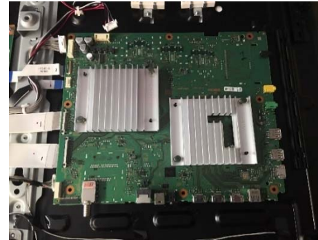
Nexus performs tear down of Television to get to target board. (Picture before attachment).
