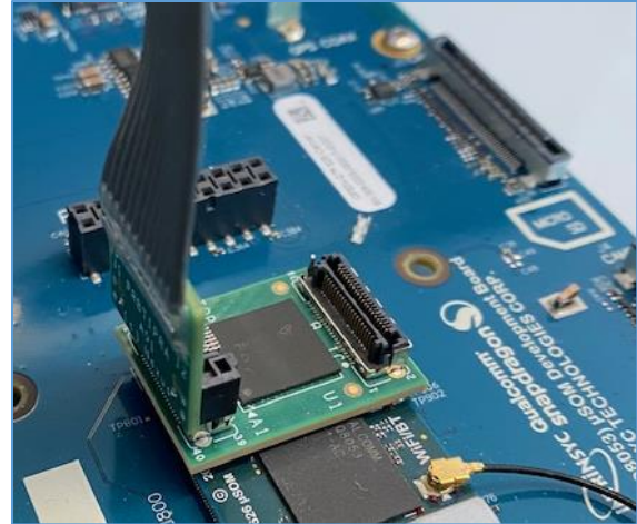
Figure 1 MA 5100 interposer installed under a memory component
