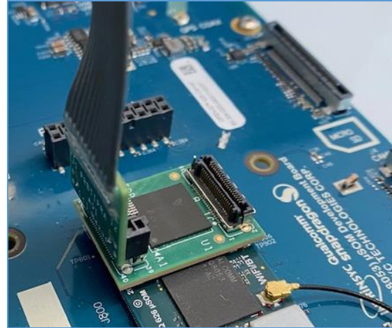
Figure 1 MA 5100 interposer installed under a memory component
