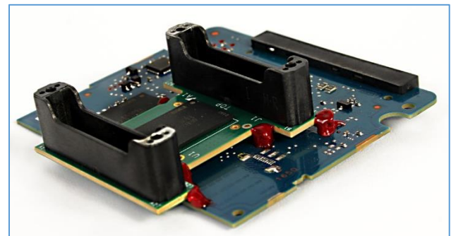
Figure 1 NAND Flash interposer installed under a memory component
