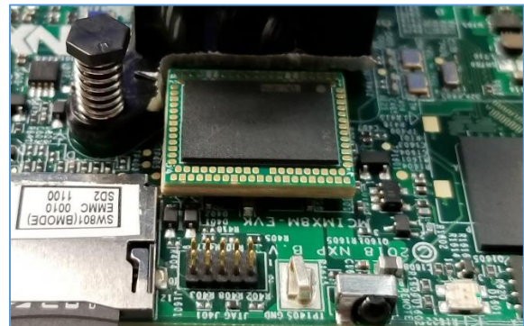
Figure 1 - Direct Attach interposer installed under a memory component
